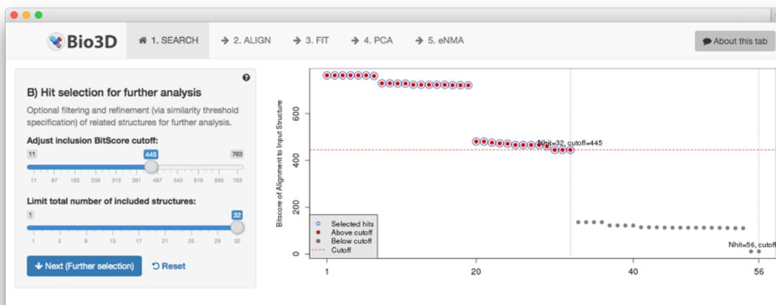
**Figure 4:** Hit selection for further analysis. The plot shows a summary of the search results where each dot represents one particular PDB ID. Dots above the dashed red line are above the specified threshold and can be selected for further analysis. Only hits marked with a blue circle are currently selected.
